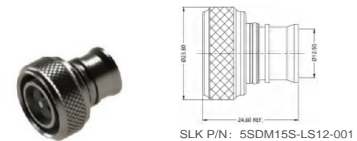
SLK P/N: 5SDM15S-LS12-001 Cable : 1/2" super flexible cable Frequency: 6 GHz
