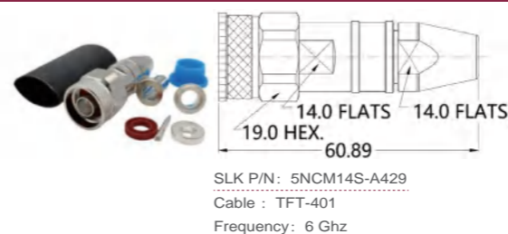
N straight male connector(Flexible cable crimping type)
