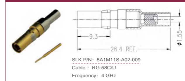
1.0/2.3 straight male connector (Flexible cable solder type)
