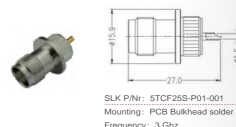
TNC straight female connector(PCB connector)
