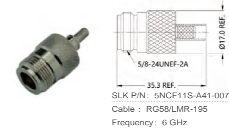
N straight female connector(Flexible cable solder type)
