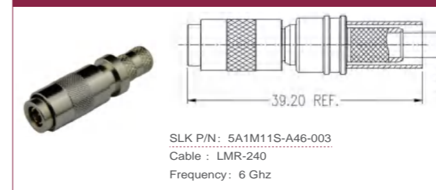
1.0/2.3 straight male connector (Flexible cable solder type)
