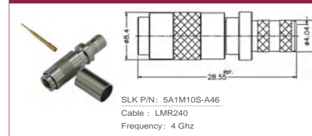
1.0/2.3 straight male connector (Flexible cable solder type)
