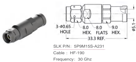
2.92mm straight male connector (Flexible cable solder type)
