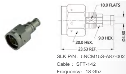
N straight male connector(Flexible cable solder type)
