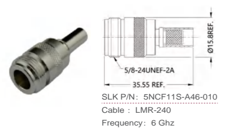
N straight male connector(Flexible cable crimping type)
