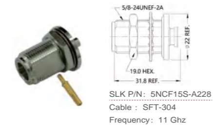
N straight female connector(Flexible cable solder type)
