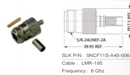
N straight female connector(Flexible cable solder type)
