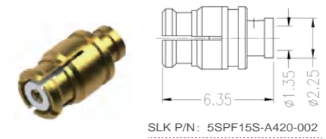
SMP straight female connector(Flexible cable solder type)
