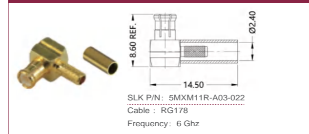
MCX right angle male connector (Flexible cable crimping type)
