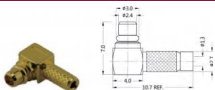
MMCX right angle male connector (Flexible cable solder type)
