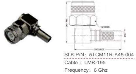
TNC right angle male connector (Flexible cable crimping type)
