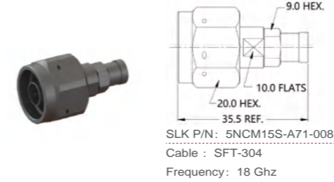
N straight male connector(Flexible cable solder type)
