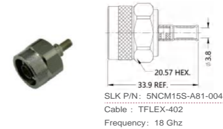
N straight male connector(Flexible cable solder type)
