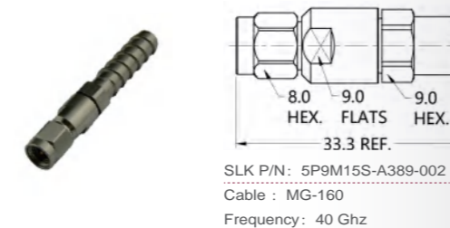
2.92mm straight male connector (Flexible cable solder type)
