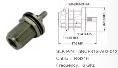
N straight male connector(Flexible cable crimping type)
