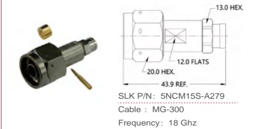
N straight male connector(Flexible cable solder type)
