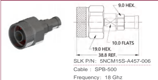
N straight male connector(Flexible cable solder type)
