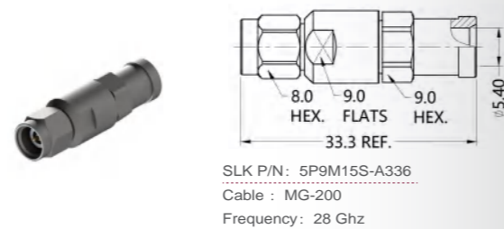
2.92mm straight male connector (Flexible cable solder type)
