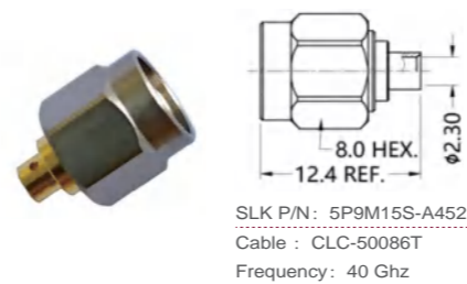
2.92mm straight male connector (Flexible cable solder type)
