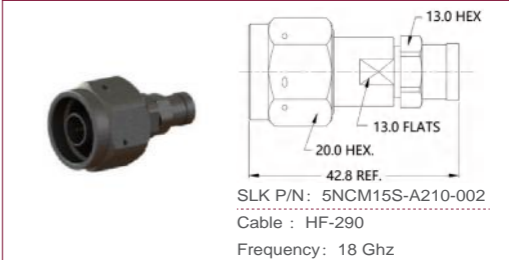
N straight male connector(Flexible cable solder type)
